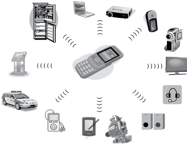
FIGURE 1.15 Bluetooth-enabled personal area networks
