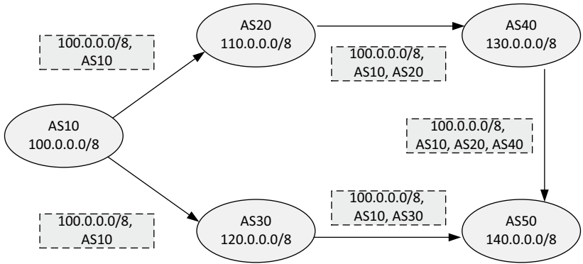
FIGURE 11.14 A demonstration of BGP mechanism
